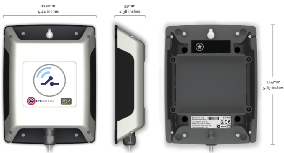
Dimensions for ZPC-10 /ZPC-20 Wireless Pulse Counter
